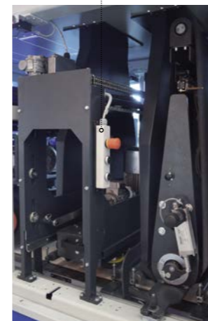
Easy zeroing of groups with internal push-button panel
